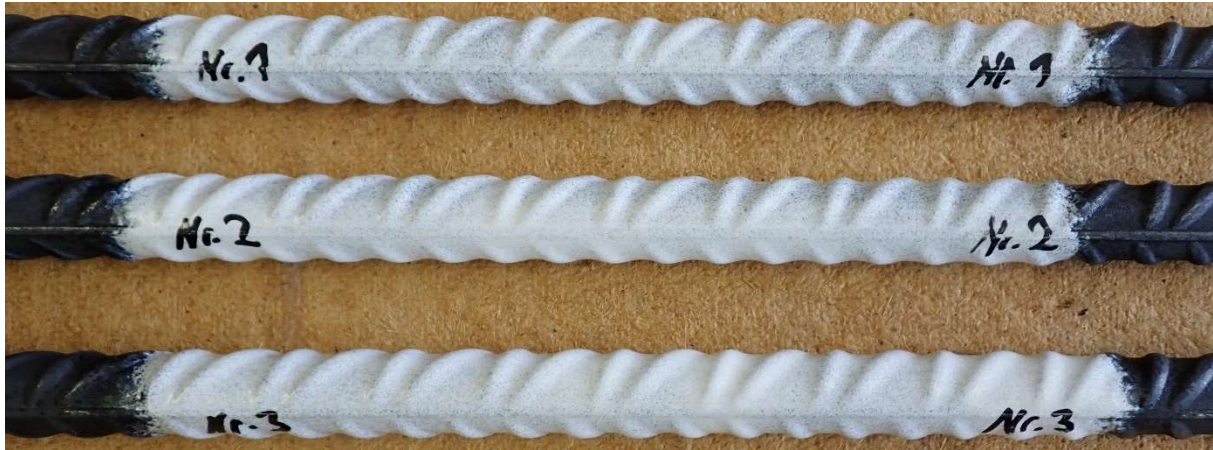
Figure 9: Opposite side surfaces of the coated anchors before NSS-test
