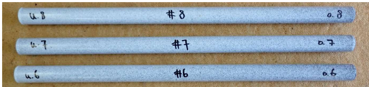
Figure 5: Opposite side surfaces of the coated dowels before NSS-test
