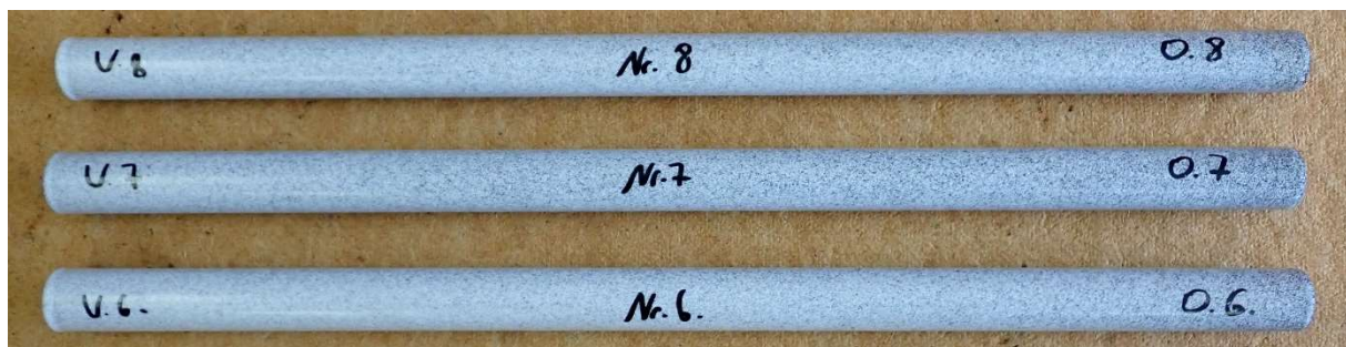
Figure 4: Dowels with plastic coating before NSS-test
