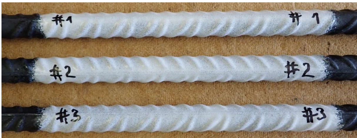
Figure 8: Anchors with plastic coating before NSS-test
